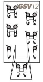
**GSV12:** This glovesheet product is designed for vertical pipes or risers up to 12' high and 12" in diameter and features a large debris chamber at the base of the sheet for waste collection. The debris area is offset from the work area, flat dimensions are 9' x 15'. 6 mil construction.
